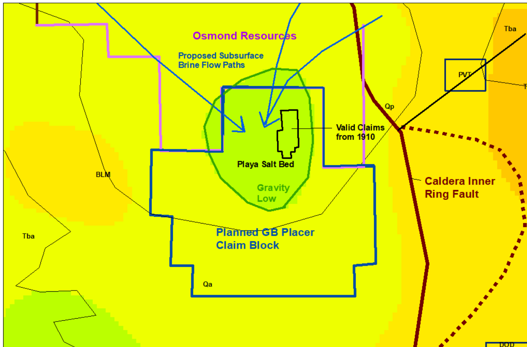
Figure 16. Salt Wells Project. Complete Bouguer Gravity Anomaly. Proposed Great Basin Lithium Corp. placer claim block - lithium brine target in gravity low below boron-lithium playa salt bed
